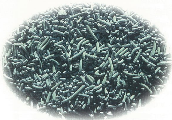
Extrudates of Hydrotreating Catalyst
