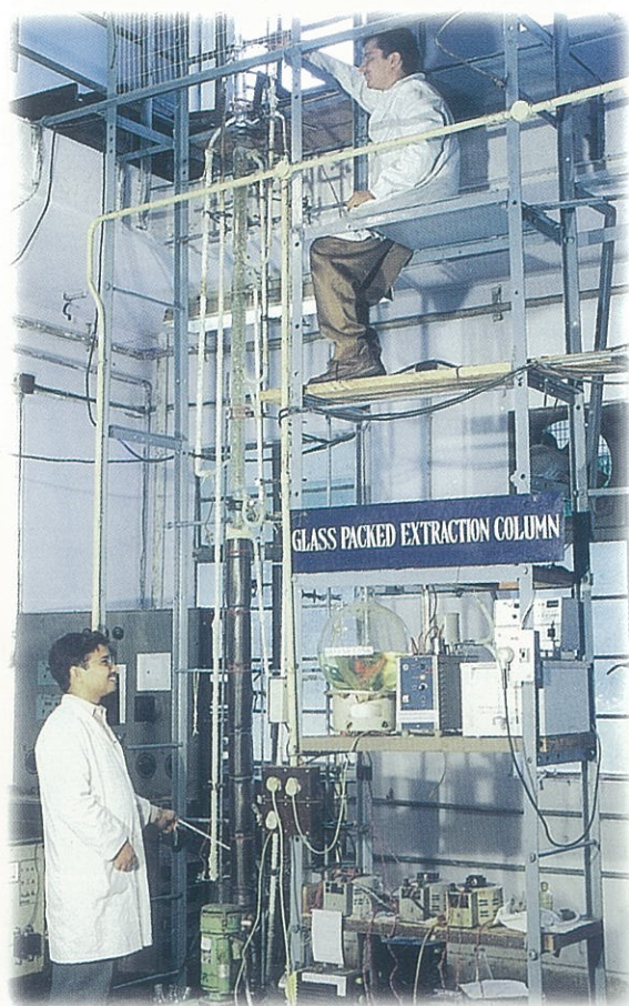
Extraction Column for Lube Studies
