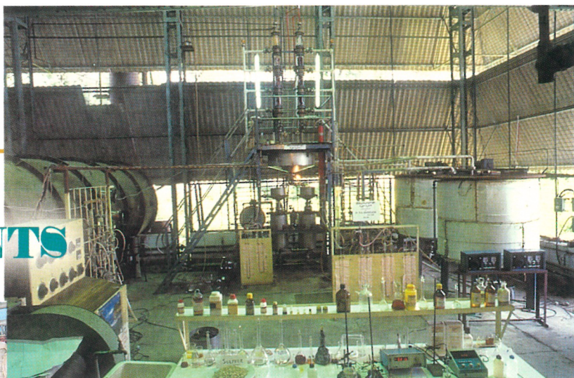
Pilot plant for desulphurisation of flue gases
